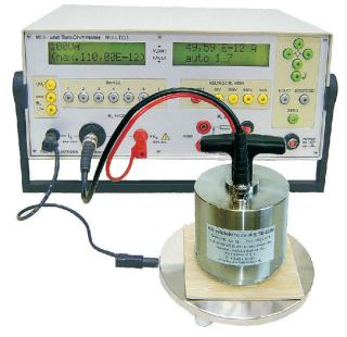
surface measurement with AE 30 and grounded base plate GP 14 (optional) connected to Milli-TO 3  $\,$
