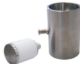
surface measurement with grounded baseplate GP 14 (optional) and Milli-TO 3 (optional)
