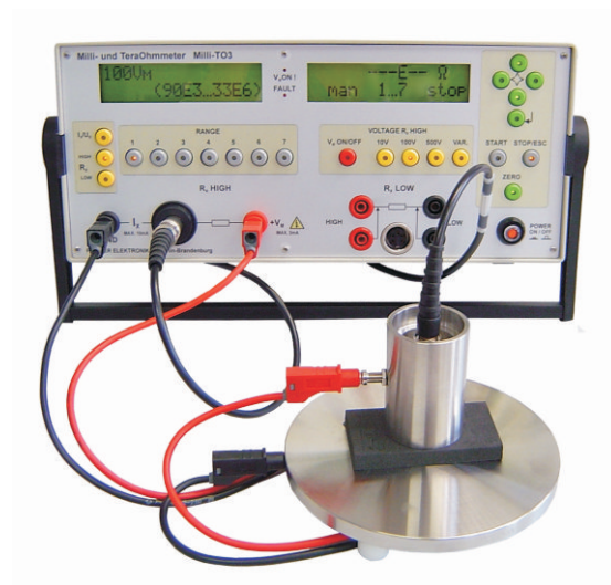
surface measurement with grounded baseplate GP 14 (optional) and Milli-TO 3 (optional)
