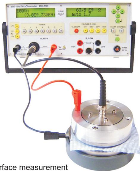
Surface measurement with grounded baseplate
