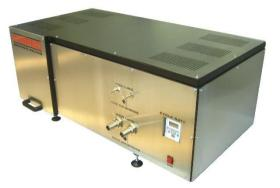
By making the appropriate adjustments to the motor controller and the mechanical drive mechanism respectively, the pneumatic cylinder is capable of providing any one of five pre-set swept volumes of 1.0, 1.5, 1.75, 2.0 and 2.5 litres at variable rates up to 40 strokes per minute.
