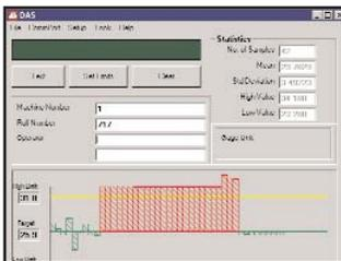
Data Acquisition Software (DAS) is a Windows® based optional software package that provides the ability to collect data and perform additional statistical analysis. DAS enables you to plot results real time against defined limits, generate semi-custom reports and export test data to other spreadsheet packages for further management.
