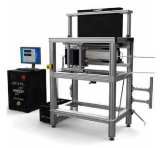
Conducting fire tests simulating the lateral spread of flames along specimens exposed to the heat of external fire. Construction products, vehicle parts (ships, trains, motor vehicles) as well as wall coverings and claddings are suitable for testing.
